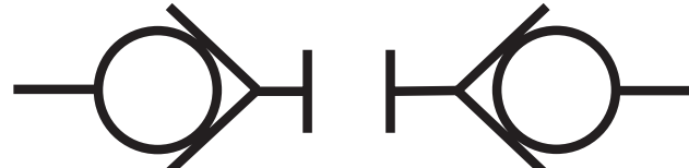
QUICK DISCONNECTS (DISCONNECTED)
