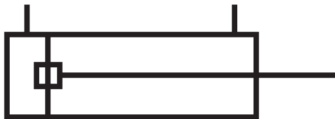
SINGLE ROD END WITH A FIXED CUSHION AT BOTH ENDS
