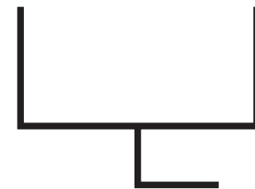
VENTED RESERVOIR SUCTION LINE ATTACHED TO BOTTOM
